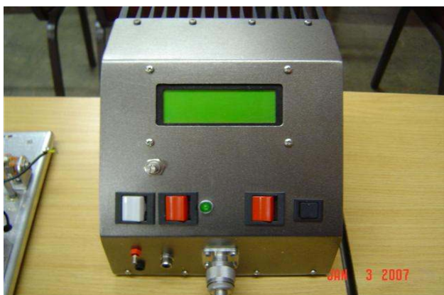
1mW – 1 kW Wattmeter with built-in two-tone generator
