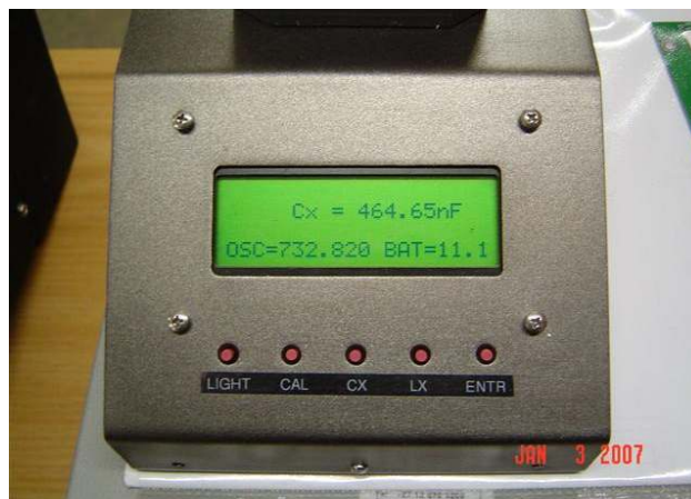
LC meter with <1% accuracy down to 15µH and 100pF
