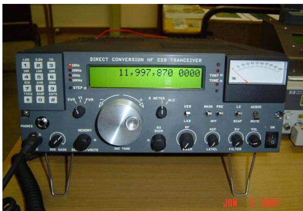
Full fledged direct conversion SSB Transceiver 220W
